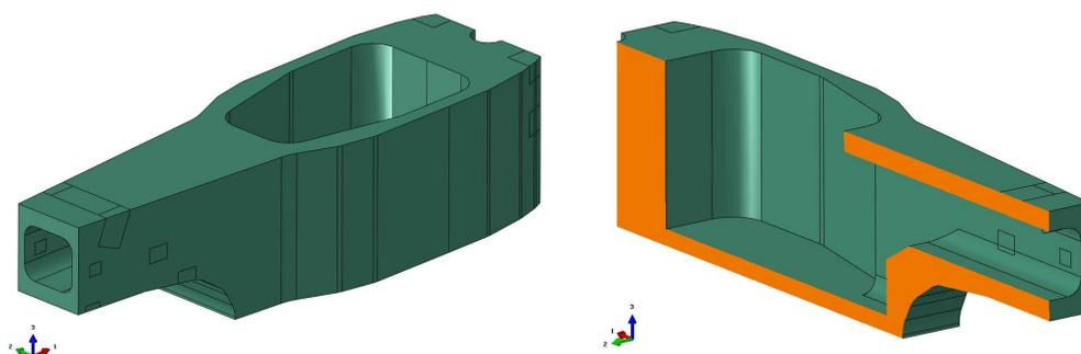
Figure 15.1. Design Space for a hypothetical single-seater racing chassis. Having imposed aluminum as a material, the mass of the Design Space is 755 kg.
