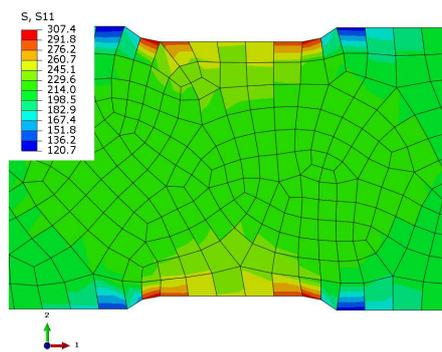
Figure 9.2. Unaveraged longitudinal stress for the coarse mesh.
