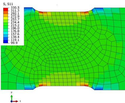
Figure 9.1. Unaveraged longitudinal stress for the fine mesh.
