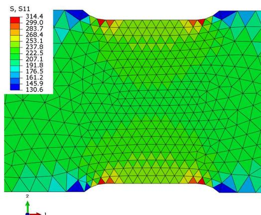
Figure 9.3. Un-averaged longitudinal stress for the mesh with triangular elements.
