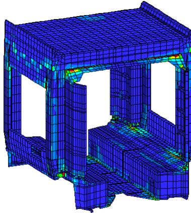
*Figure 27. Central car body shell for a tramway vehicle. Aluminum extruded beams and panels bolted and riveted together.*
