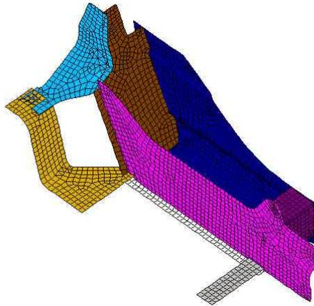
*Figure 28. Lift truck frame (only a half is represented here): welded steel plates.*
