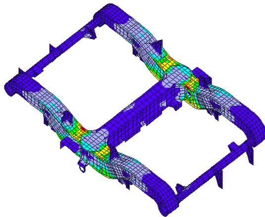
*Figure 26. Railway motor bogie. The structure is obtained by steel plates cut and welded together.*
