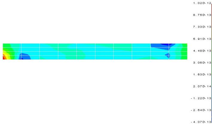
Figure 3. Vertical stress contour when the constraint distribution has been modified. Now the vertical stress value along all the domain is practically null. Its order of magnitude is  $10^{-12}$ .
