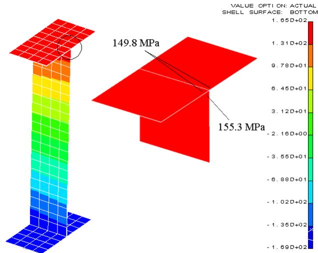
Figure 16. Non averaged longitudinal stress in the middle section of the beam: bottom faces. An enlarged portion of the model is reported in order to illustrate the stress values, in the interface node, for the web and flange elements.
