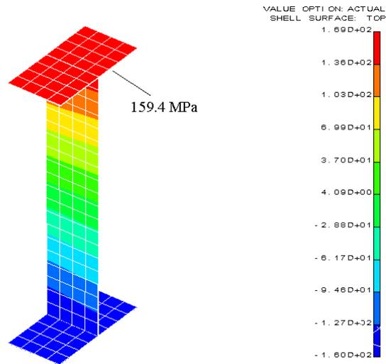
Figure 14. Longitudinal stress in the middle section of the beam: top faces.
