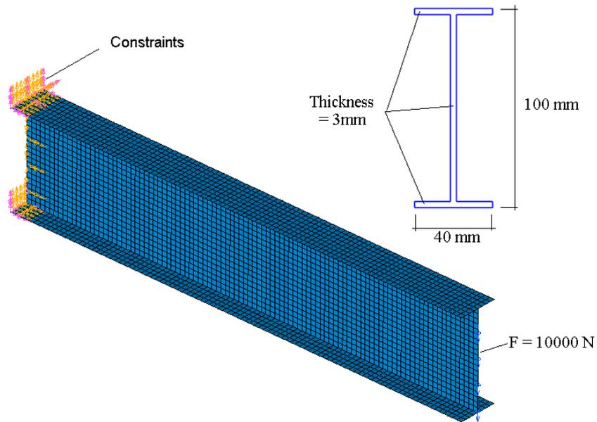
Figure 12. The beam has a length  $L = 500 \text{ mm}$ . Shell elements lie in the middle planes of web and flanges.
