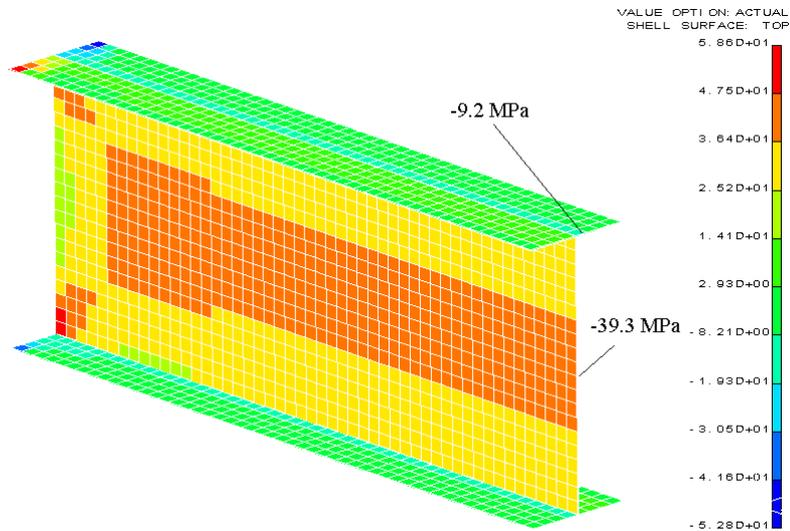
Figure 17. Shear stress contour. Both in the web and the flanges the agreement between theory and finite element model is very good
