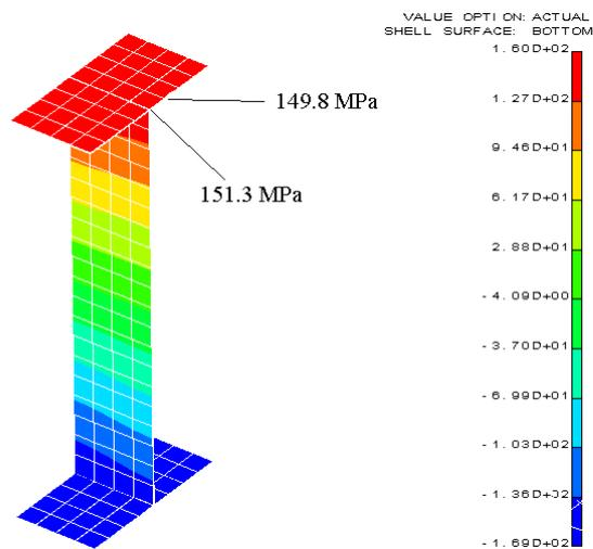
Figure 15. Longitudinal stress in the middle section of the beam: bottom faces.
