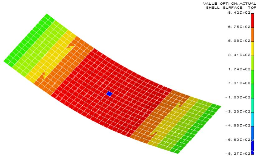
Figure 11. Non averaged stresses in longitudinal direction. It is possible to notice the discontinuity due to the presence of an upside down element.
